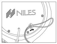
Figure 8 Security Cable in Eyelet
